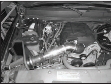
Step 21 Reinstall the engine cover. Make sure that all clamps and hardware are fully tightened. Reconnect the battery cable, start the vehicle and let it warm up. Shut off and inspect the installation once more for any loose clamps, wires, or hardware. Test drive & enjoy! Your installation is now complete. Periodically check all clamps and brackets.
