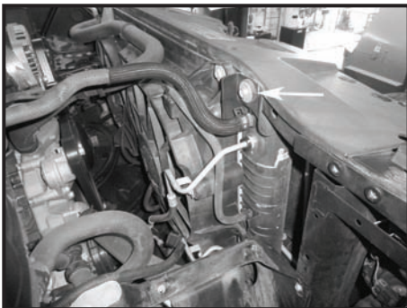
Step 12 Remove the bolt from the radiator shroud. This will be reused in Step 14.
