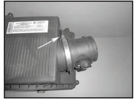
Step 9 Remove the MAFS from the factory air box making sure the factory boot stays on the MAFS.
